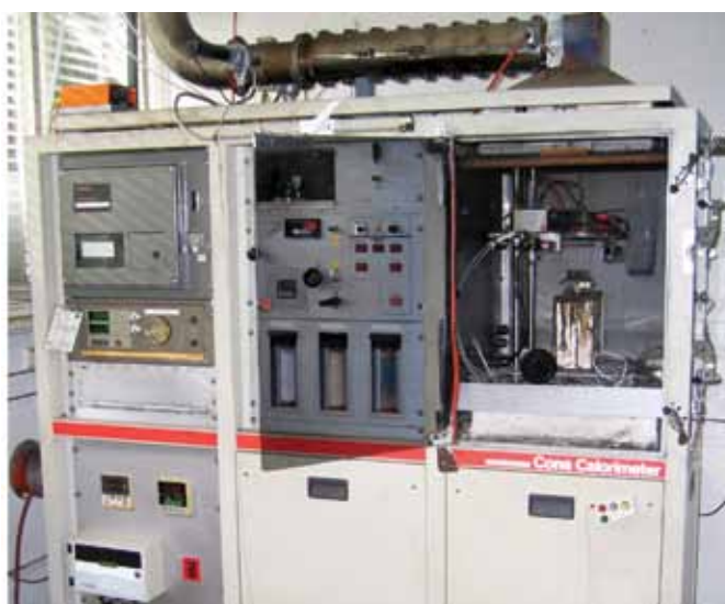
◀ The cone calorimeter is a small-scale fire test apparatus designed to measure rate of heat release, mass loss rate, ignitability, smoke density and gas species production rate.
