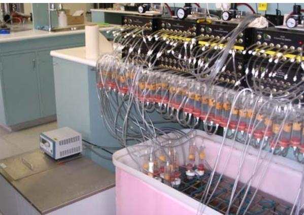
Soil respiration measurements were taken using a system whereby O<sub>2</sub> uptake as well as CO<sub>2</sub> efflux can be measured dynamically. Using an open flow system combined with a differential oxygen analyser (DOX) and an Infra Red Gas Analyser (IRGA), we can quantify respiratory quotients as well as rates of respiration.
