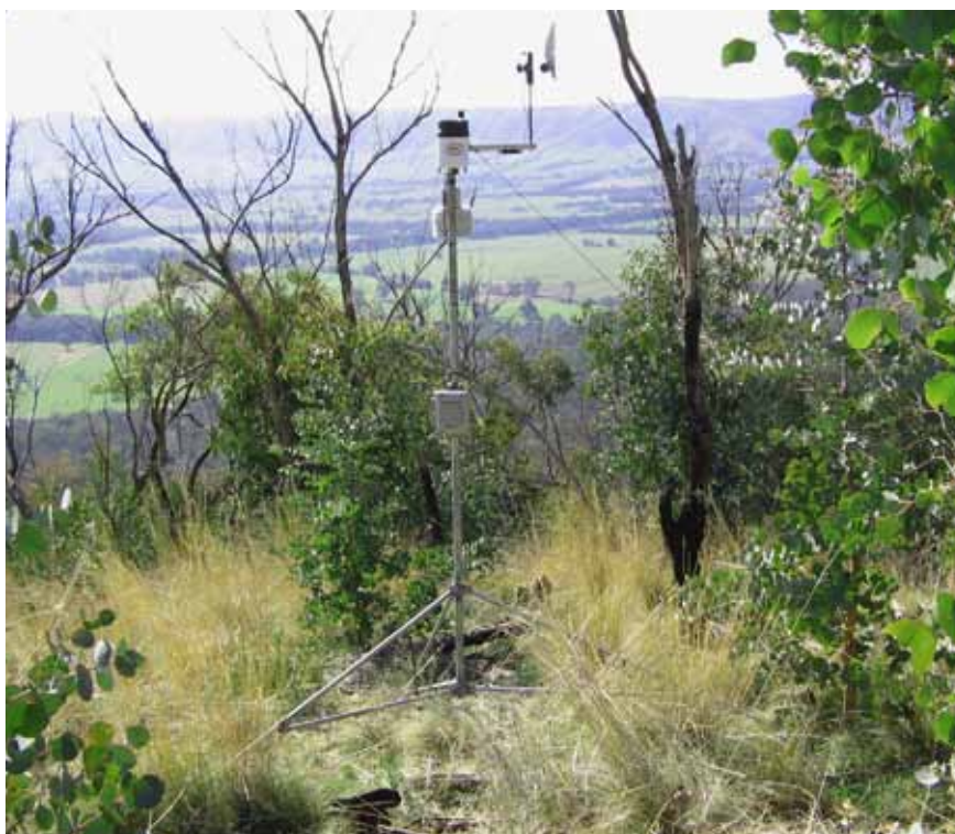
▲ Figure 1: Micro-metrological stations were set up at research sites in north east Victoria to enable continuous measurements of the environmental variables that drive water use by plants.
