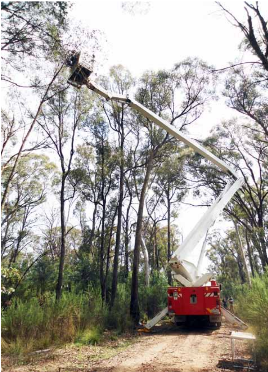
▲ Figure 2: An old fire truck with a cherry picker allows researchers to easily access leaves from the canopies for measurements.
