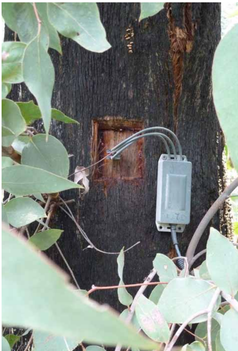
▲ Figure 3: Sensors measure the rate of movement of water through a stem.
