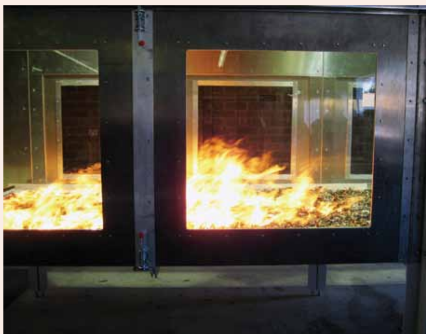
▲ An experimental fire burning in the CSIRO Pyrotron in Canberra. The facility allows free-burning fires to be studied under repeatable conditions in safety.
