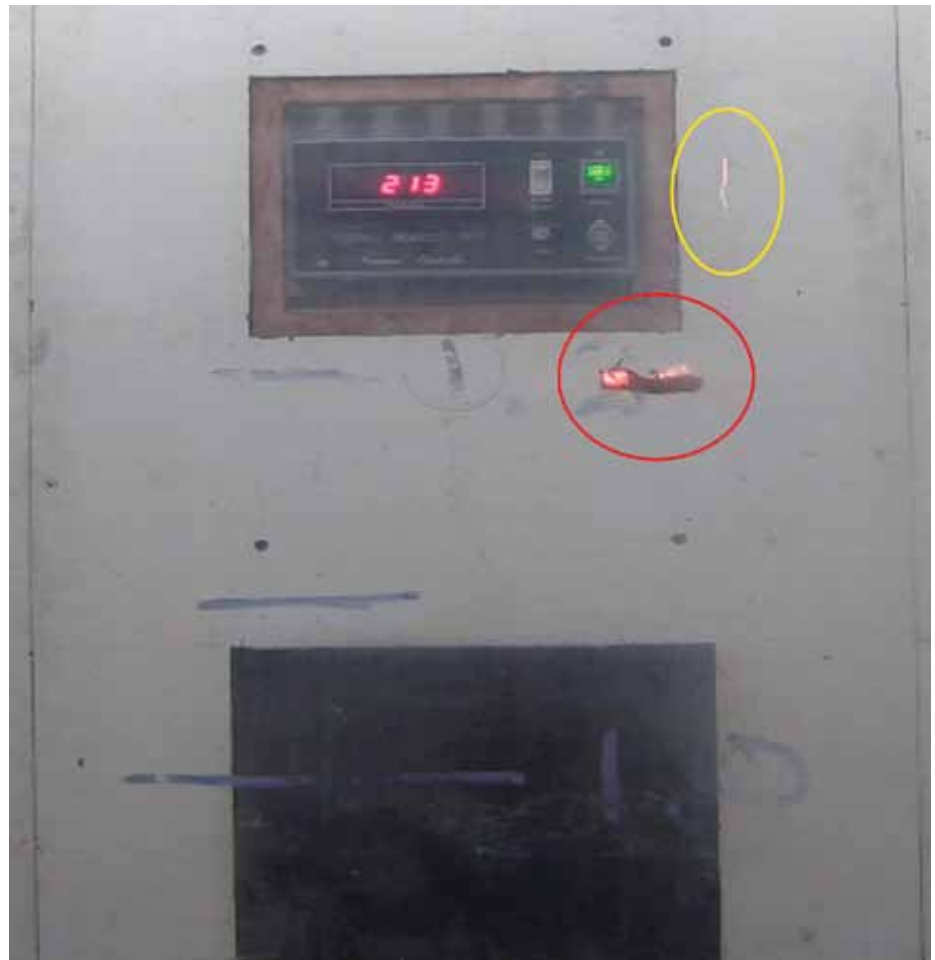
▲ A eucalypt bark firebrand (circled in red) being studied falling at its terminal velocity while it burns in the CSIRO Vertical Wind Tunnel. An ember (circled in yellow) has broken off the firebrand and is being accelerated away in the air stream.
