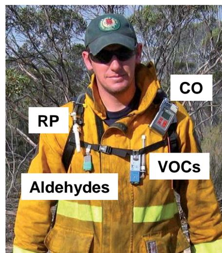
▲ FIGURE 1: FIRE FIGHTERS FITTED WITH PERSONAL SAMPLING DEVICES
