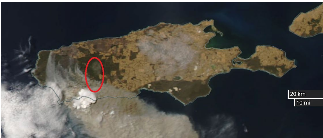
FIGURE 4. MODIS CORRECTED REFLECTANCE (TRUE COLOUR) IMAGERY FROM JANUARY 2ND, 2020. THICK SMOKE OBSCURED THE INFARED SIGNAL AFFECTING BOTH MODIS AND AHI ACTIVE FIRE PRODUCTS. THE LARGEST DATA GAP IS WITHIN THE RED ELLIPSE. SOURCE: EOSDIS WORLDVIEW.
