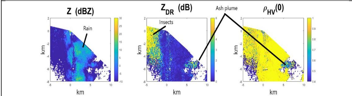
Fig. 10 Sector scans on 8/5/2022 illustrating the ability of the radar to separate out clear air (insect) echoes, moderate rain and a small ash plume from a local burn.
