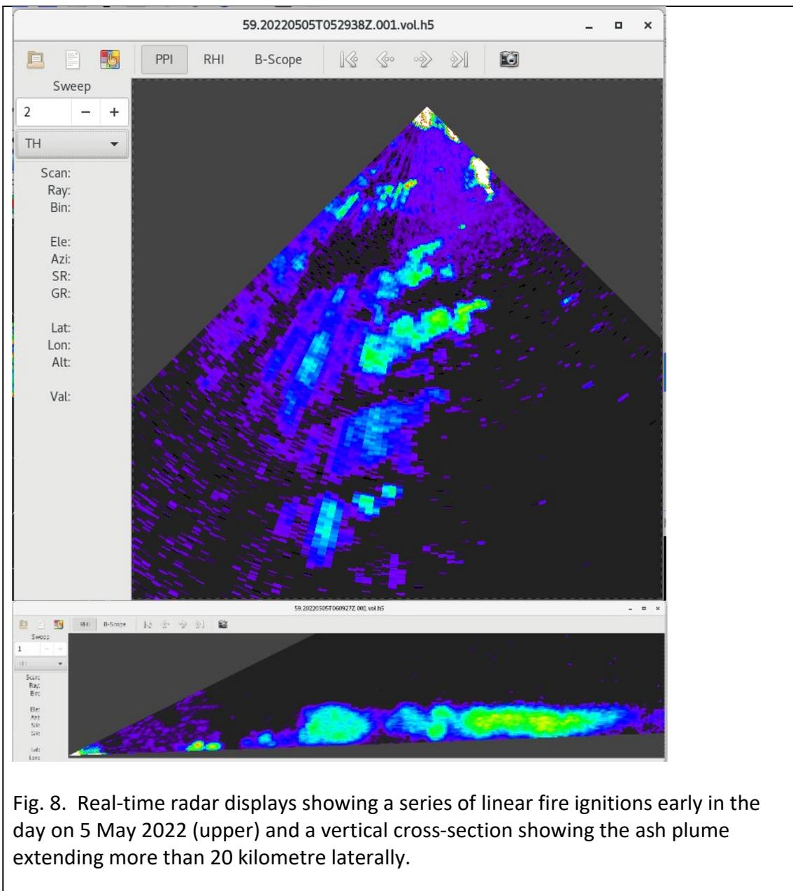
Fig. 8. Real-time radar displays showing a series of linear fire ignitions early in the day on 5 May 2022 (upper) and a vertical cross-section showing the ash plume extending more than 20 kilometre laterally.
