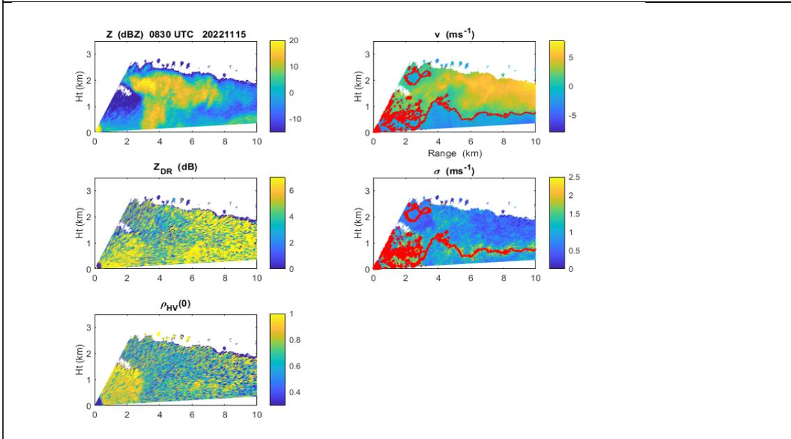
Fig. 11 Vertical cross-sections of an intense column on 15 November 2022 showing clear air echoes close to the radar, the column feeding the downwind plume and an approaching sea breeze feeding the inflow into the column. The spectral width shows enhanced turbulence at the top of the sea breeze in the region of maximum shear.
