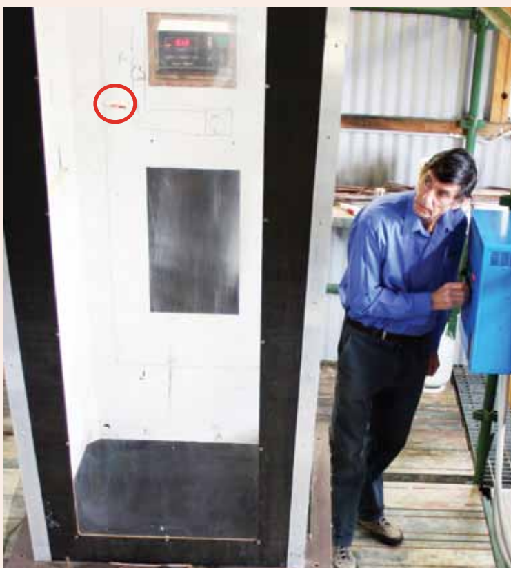
▲ Dr Peter Ellis demonstrates how the CSIRO vertical wind tunnel allows untethered firebrand samples (circled) to be burnt at their terminal velocities in the laboratory, as though they were actually in flight. This is convenient for taking measurements and observations.
