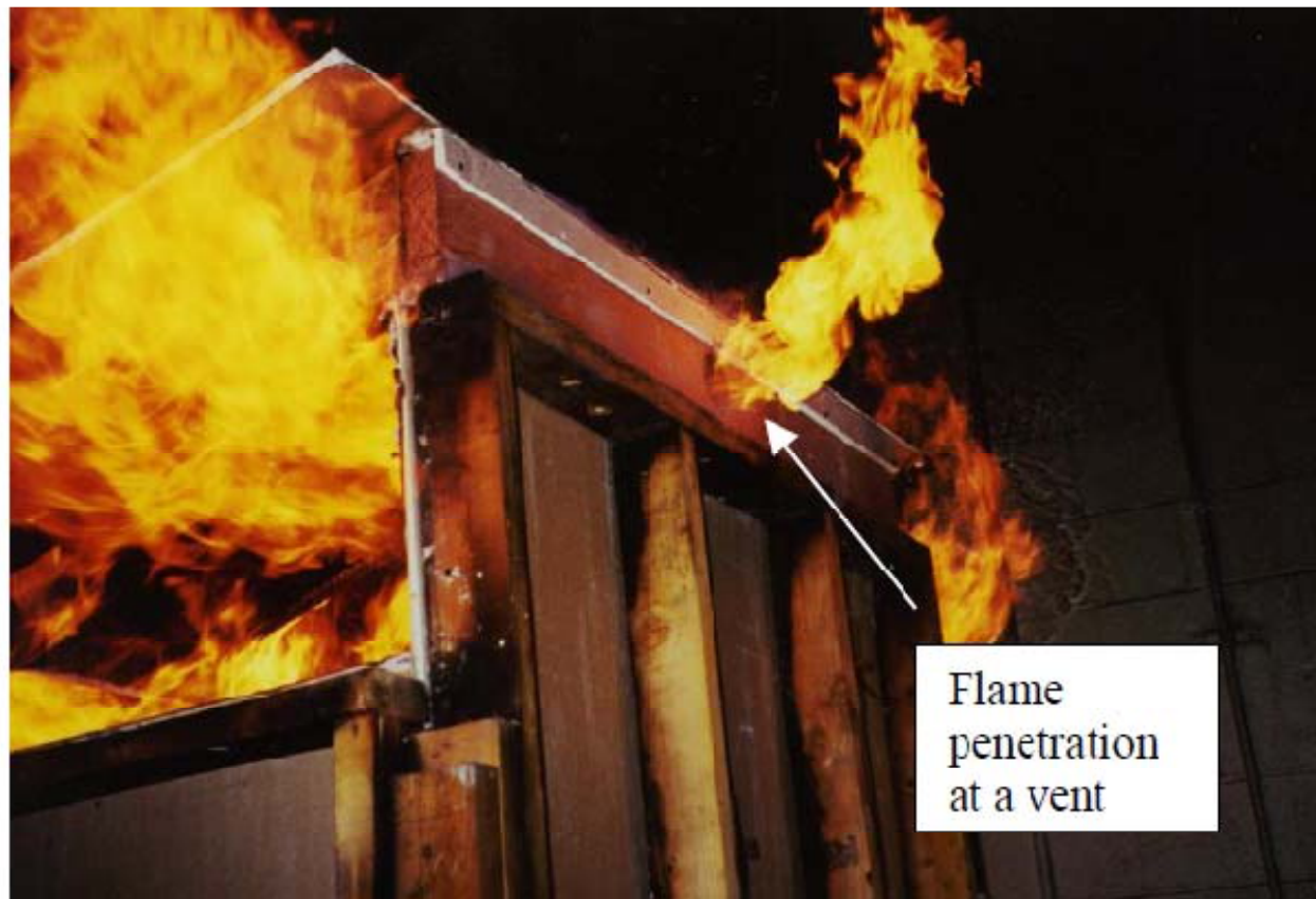
Figure 1. This photograph shows flame penetration through a 2-inch diameter soffit vent located in the center of the wall, as viewed from what would be the interior of a structure. The flame impingement exposure simulates burning vegetation or exterior cladding.
