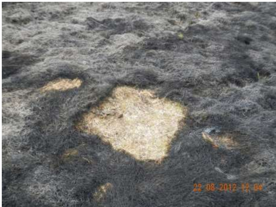
Figure 6. Unburnt fuel quadrat ( 1\text{m}^2 ) after the burn in Phalaris dominated grassland at Fraser. Five quadrats were taken from each replicate to determine the fuel load. All fuel was removed from the quadrat and dried at 105^\circ\text{C} for 24 hours to determine the oven-dried weight.
