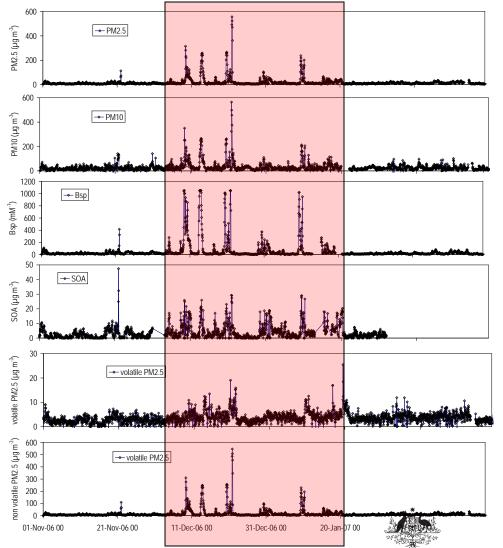
Time series of hourly concentrations of PM2.5, PM10, Bsp, SOA, volatile PM2.5 and non-volatile PM2.5.
