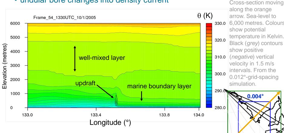
along the orange arrow. Sea-level to 330.0 6,000 metres. Colours show potential temperature in Kelvin. Black (grey) contours show positive 310.0 (negative) vertical velocity in 1.5 m/s intervals. From the 0.012°-grid-spacing simulation.
