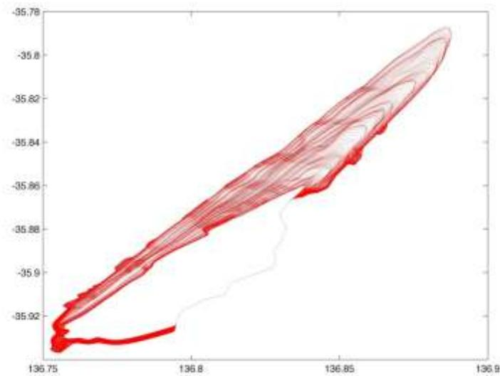
**Figure 3.** Fire isochrones for the Rocky River fire at one-minute intervals. Simulation from 0600UTC to 0830UTC.
