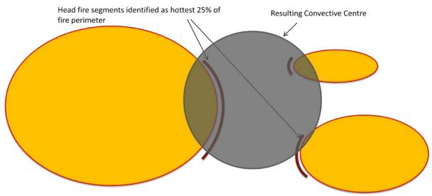
Figure 1. Fire perimeter 'hottest' segments (brown arcs) are identified then aggregated where appropriate to form a convective centre (grey circle).
