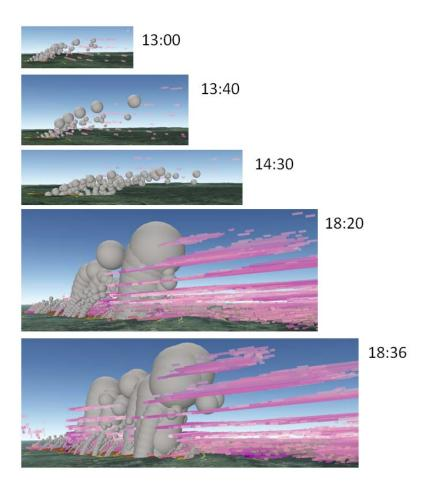
Figure 6. South-easterly run of the Kilmore fire showing modelled plume bubbles as white spheres compared to radar reflectance scans indicating smoke location and density in pink.
