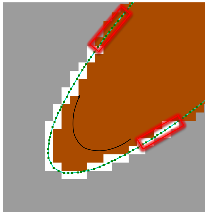
Figure 1. Fire perimeter is shown in green with dots representing the vertices. White pixels indicate a section that has been identified as being in the top 25% of perimeter intensities. The running 10 point average shown in red has traversed the perimeter, entering and exiting the 25% threshold value.
