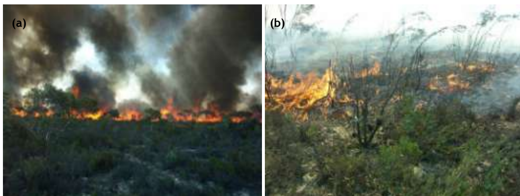
FIGURE 3.2. (a) Western head/flank corner of plot AS1 fire at 14:43:50 with flames up to 2 m. (b) Fire behaviour in drop G2 footprint at 14:47:44, 3 minutes after the gel suppressant drop, with residual flames around 0.2 m.
