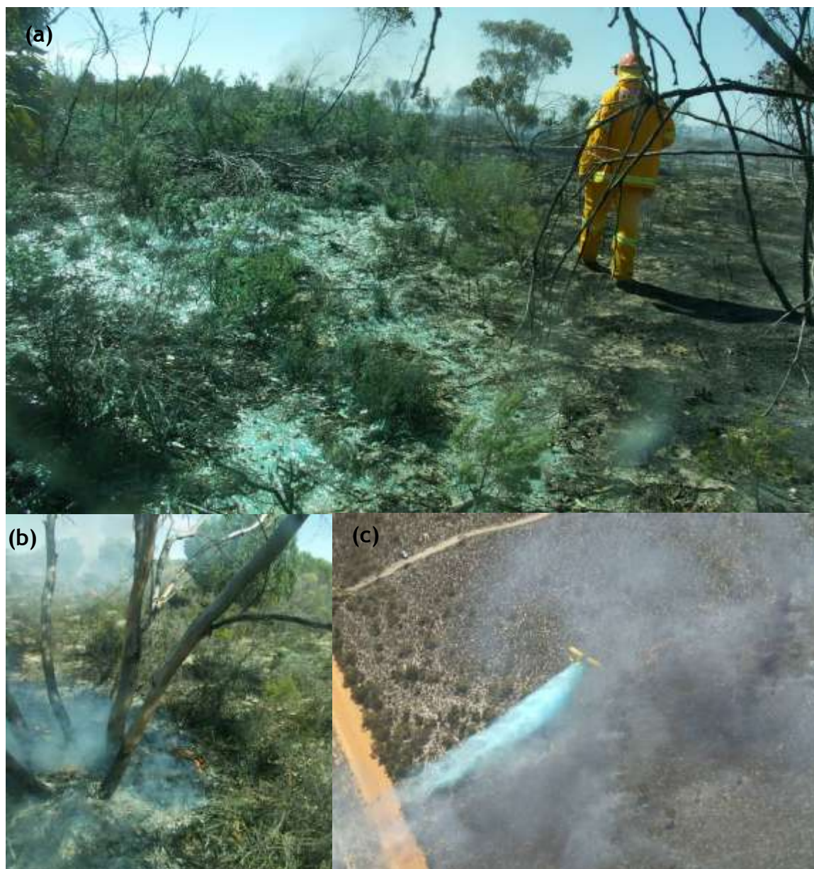
FIGURE 3.3. (a) Thick coverage of drop G8 with apparent full extinction of flank fire 7 minutes after drop. (b) Small residual flames ( <0.1 m) in a section of lighter coverage 10 minutes after drop. (c) Aerial view of the drop being made on the western flank.
