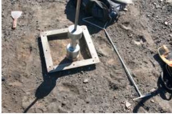
Figure 3. Heavy duty square sampling frame, soil bulk density corer and extraction handle developed for accurate sampling of forest floor carbon before and after fire.
