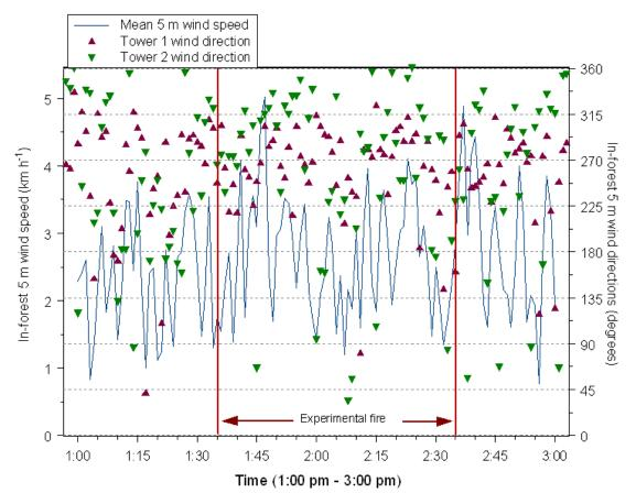
**Figure 7.3:** In-forest mean wind speed and wind direction from two sonic anemometers at 5 m at Bungongo Plot D1 experimental fire.
